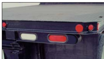
Horizontal mounting under chassis frame
