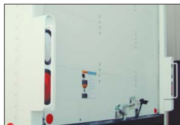
Vertical mounting on rear corner posts of truck body
