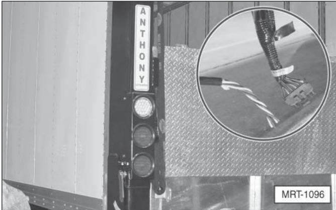
5. Attach the license plate and license plate light to the chassis (or trailer) below the level of the truck floor using the original bracket.
