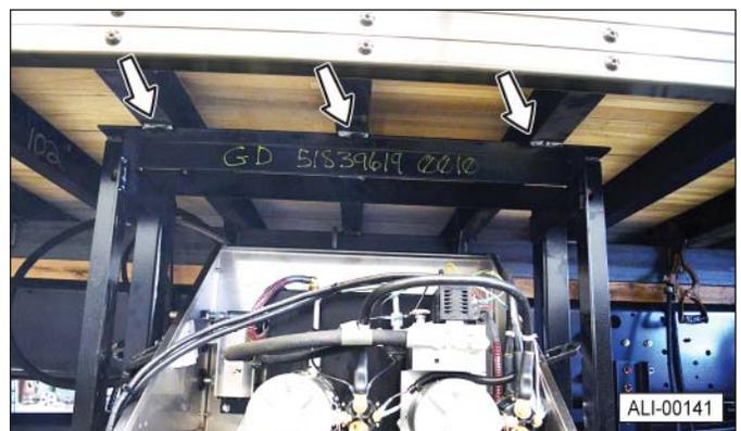
4. Raise the battery box unit until the “hanger channel” contacts the underside of the chassis (or trailer) crossmembers.
