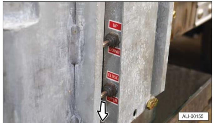
6. Raise and lower the platform to make sure it operates without binding. Air introduced into the system during installation will work itself out after several cycles of normal operation. To bleed air out of the cylinders, refer to "4.12 Air Bleeding Procedure For MRT Liftgates (Gravity Down Models ONLY!)" on page 30.
