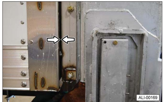
9. Tack weld the liftgate to both corner posts of the vehicle. Place the tack welds (8 welds) at the top and bottom (inside and outside) of each column. The tack welds should be a minimum of 3/16 x 2 inches long and capable of holding at least 2600 pounds.
