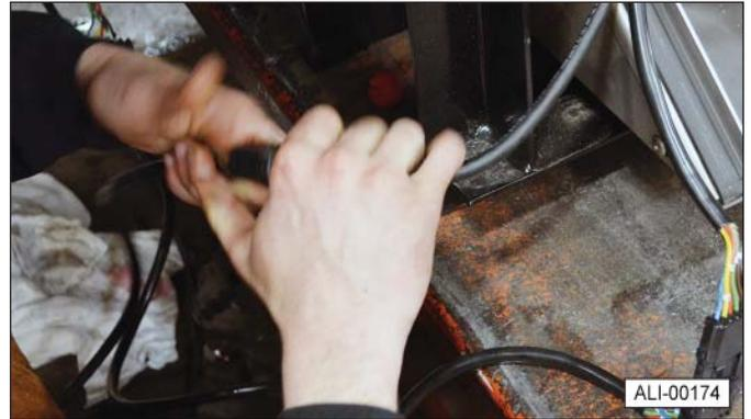
12. Connect the liftgate tail light cable, which controls the running lights, backup lights, and brake lights, to the truck wiring harness.
