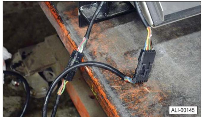
13. Use clamps or plastic ties (provided) to secure the hoses and wires to the crossmembers, approximately every three feet.
