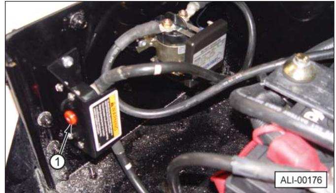
Circuit breaker in vehicle battery box.
