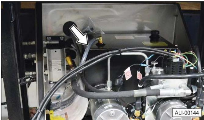
10. Route the liftgate control cable through the split grommet in the back of the power pack enclosure.
