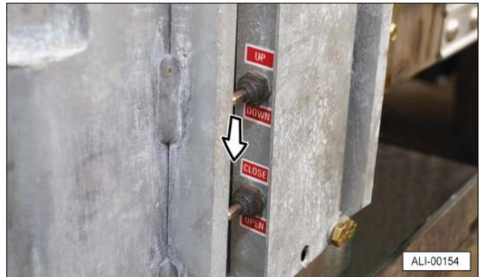
5. Press the Open switch to unfold the platform.
