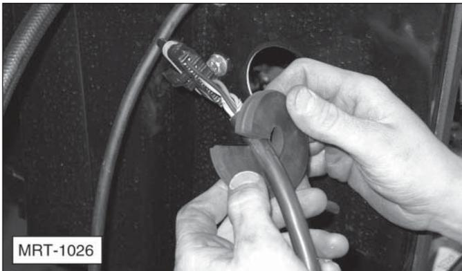
11. Connect the liftgate control cable, which controls all the liftgate functions (up, down, open, and close) to its mating connection inside the power pack enclosure.
