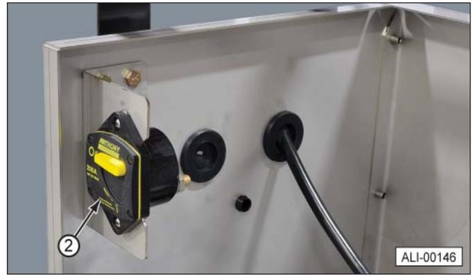
Circuit breaker in liftgate battery box.
