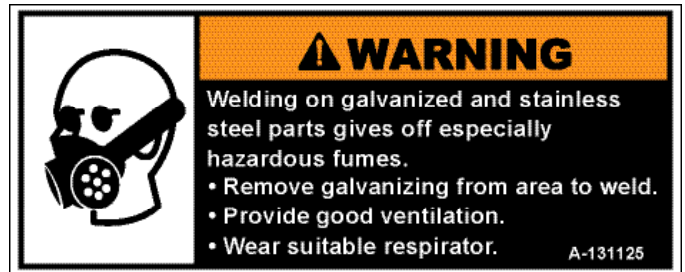
12 — A-131125 (galvanized liftgates only)
