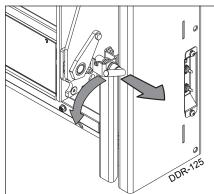
To stow the liftgate platform, first release the spring-loaded platform lock by pulling outward and rotating until the spring pin is securely in the lock notch. Then close the platform and run upward until it is latched in the column latches."
