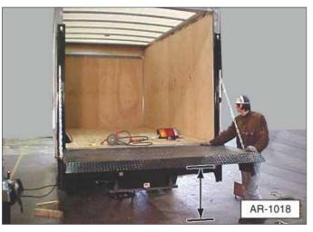
17. Install lights or other electrical components, if needed. The RailTrac Liftgate has "knock outs" for the tail lights and backup lights. Simply remove the steel plug(s) and install the light(s). Also install a license plate holder.
