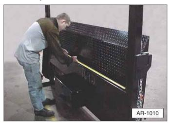
2. Measure and determine the centerline of the truck's rear sill. Mark this point.
