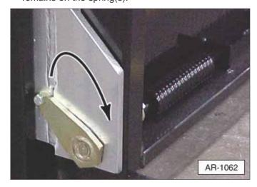
5. Loosen any setscrews that secure the spring, then remove the spring and torsion bar.
