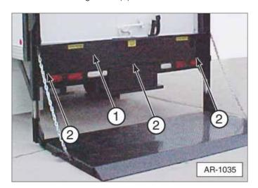
3. Calculate the proper length of chain to be removed (if any) using the formula below, if the truck bed is between 28" and 49". If the truck bed is between 50" and 58", no chain removal is required.
