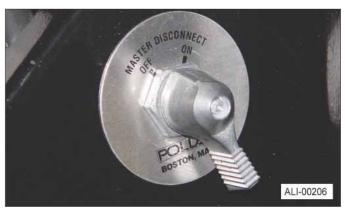
Cut-off switch mounted in cab of truck.
