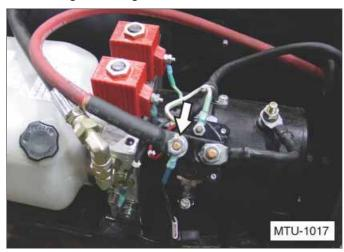
Connect power cable to motor solenoid.
