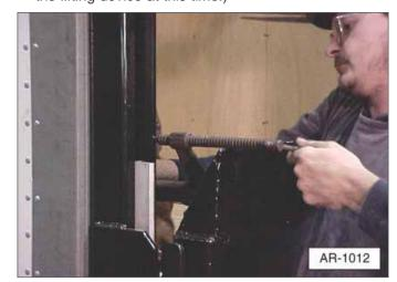
5. Tack weld the liftgate's H-frame columns to the truck's side rails and the housing to the truck's rear sill. Make sure the tack welds can hold at least 800 pounds.
