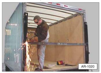
14. Cut a diagonal support brace and weld it to each H-frame column.
