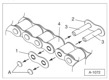
Grind heads (A) from chain link pins (3). Remove front link (1) and push rear link (2) with chain link pins (3) out.
