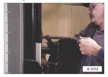
Tack weld the liftgate's H-frame columns to the truck's side rails and the housing to the truck's rear sill. Make sure the tack welds can hold at least 800 pounds.
