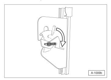
Latch shown in "released position", ready to lower and open platform.
