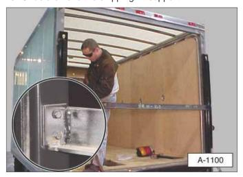
16. Cut a diagonal support brace and weld it to each H-frame rail.
