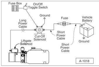
Wiring diagram with cut-off solenoid.
