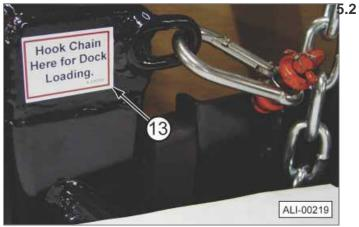
13. Hook Chain Here for Dock Loading (A-131078) **-Factory Installed-**
