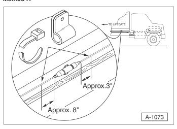
Fasten the power cable to the truck body. Locate one fastener (battery side) within 3 inches of the end of the fuse assembly. Locate the other fastener (power unit side) within 8 inches of the fuse assembly.
