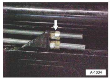
Recheck the side-to-side levelness of the platform to the truck bed. Re-adjust the platform leveling nuts, as necessary.
