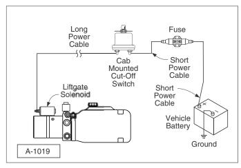
Wiring diagram with cab cut-off switch.
