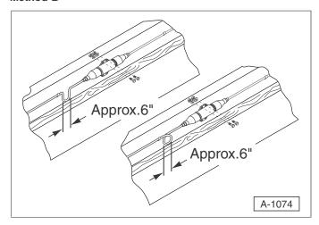
Attach the fuse holder to the truck body longsill using #10 or #12 self-tapping screws or bolts, washers, and self-locking nuts. Fasten the power cable, as needed, to properly hold it in place. Using this method requires an extra length of cable on one side of the fuse assembly to permit removal of the fuse.
