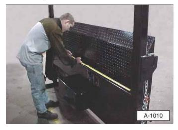
Measure and determine the centerline of the truck's rear sill. Mark this point.
