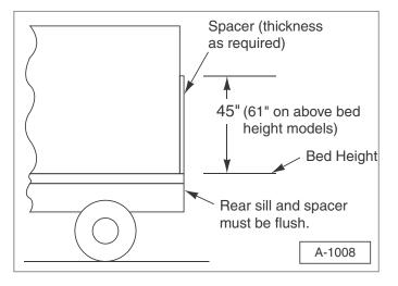
7. Weld the spacers to the corner posts using 3/16 x 2 inch long welds every 12 inches.
