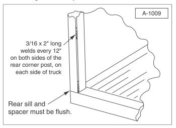
**Note**: An alternative to one long spacer is using 3 inch long plates spaced 9 inches apart. Make sure the last plate is located 45 or 61 inches above the bed height, depending on the liftgate model being installed.
