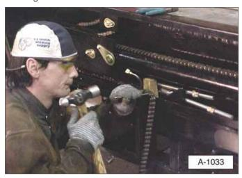
**Note**: Using a chain link removal tool will greatly reduce the time spent removing these links. These tools are normally available at motorcycle shops or other chain component suppliers.
