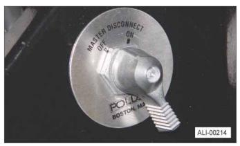
Cut-off switch mounted in cab of truck.
