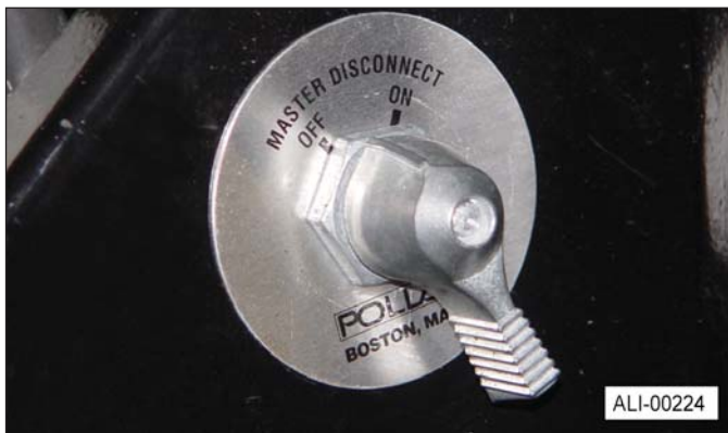
Cut-Off Switch Mounted in Cab of Truck.
