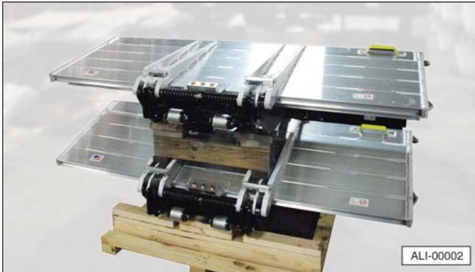
Typical Multiple Liftgate Shipping Pallet (aluminum liftgates shown).
