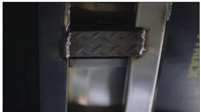
5. Weld and/or bolt the side gussets to the dock bumper and the truck body. If welding to the truck body cross-members, make sure it spans at least three of them.
