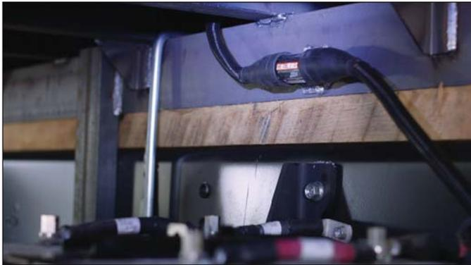
13. Route the short, 3 foot section of cable into the battery box and connect the end to the positive (+) post of the truck battery.
