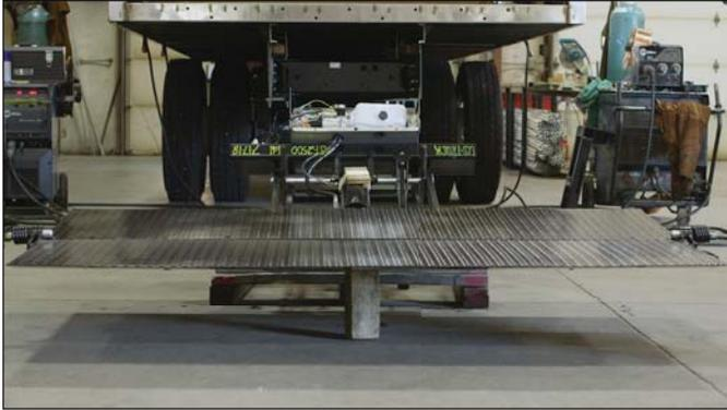
**Note:** A spacing guide is installed over the end of the cylinder rod. Do not remove this guide until the liftgate has been tack welded in place on the truck body.
