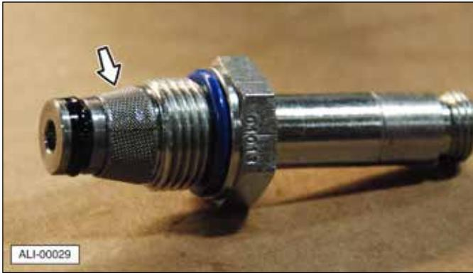
If the solenoid is working electrically, check the debris screen and clean if dirty.
