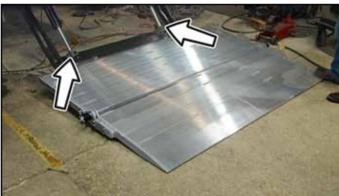
15. The front edge of the flip-over platform section should lower to the ground and contact the ground at the points as shown, and the back of the platform should raise flush to the floor extension. If the front edge does not touch the ground, refer to the next step.
