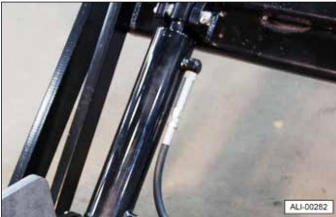
If the cylinder does not operate or operates slower than normal, remove the flow control valve and hook the hydraulic hose directly to the cylinder. If the cylinder operates properly, replace the flow control valve.
