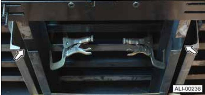
2. Insert the walk ramp cage between the long sills of the truck body. Do not secure the cage at this point.
