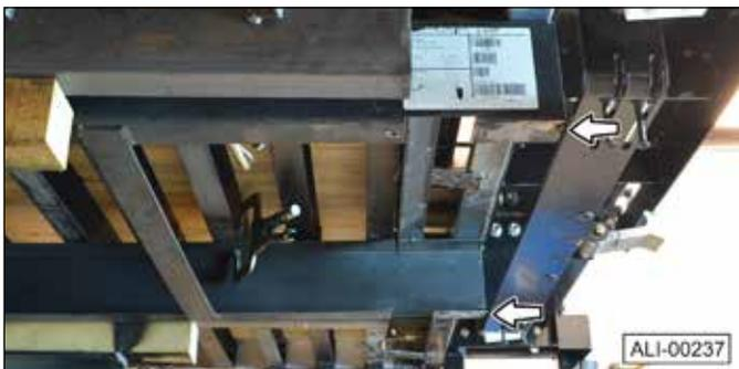
**Important:** Make sure the walk ramp cage does not hang below the walk ramp support box.
