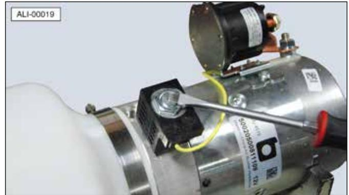
3. Momentarily activate the control switch in the DOWN position. The screwdriver should be attracted to the magnetic field created by the solenoid.
