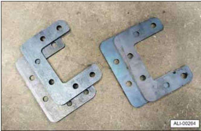
3. To adjust the width, remove the six bolts and nuts from each mounting plate. Add or remove spacers to achieve the desired width, and replace the bolts and nuts. Be sure to make the same adjustment on both sides to keep the liftgate centered.
