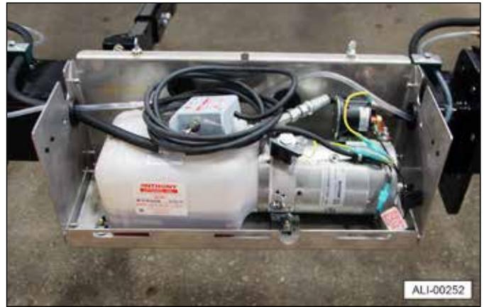
**Note:** The power unit box should contain the power cable and switch, plastic tie wraps for the battery cable, and one package containing decals, shims, a 200 Amp fuse, and manuals.
