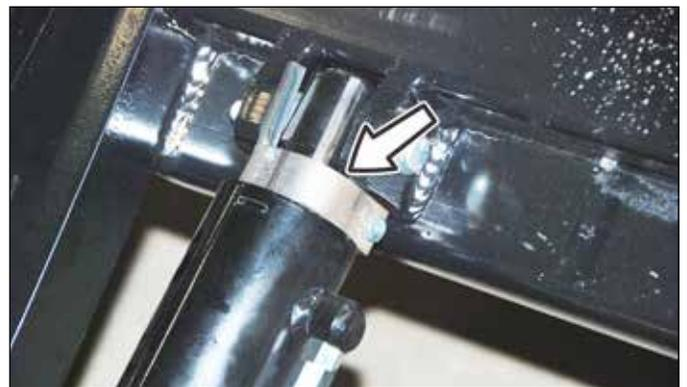
5. If necessary for liftgate clearance, cut the chassis frame and body long sill, as shown in the following illustration. After making the cut, make sure the liftgate operates properly without interfering with the chassis frame or body long sill.
