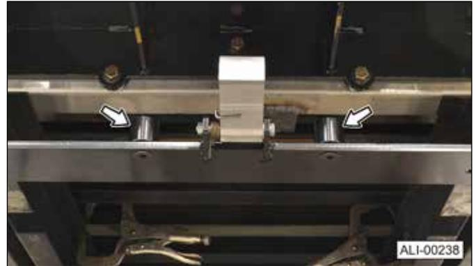
**Note:** The walk ramp stops may be left out if other methods of ramp retention are used.
