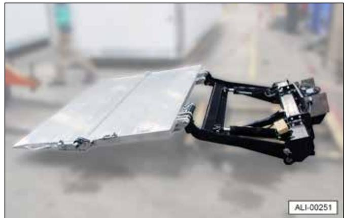
**Note:** A spacing guide is installed over the end of the cylinder rod. Do not remove this guide until the liftgate has been tack welded in place on the truck body.
