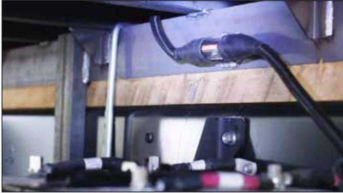
14. Route the short, 3 foot section of cable into the battery box and connect the end to the positive (+) post of the truck battery.
