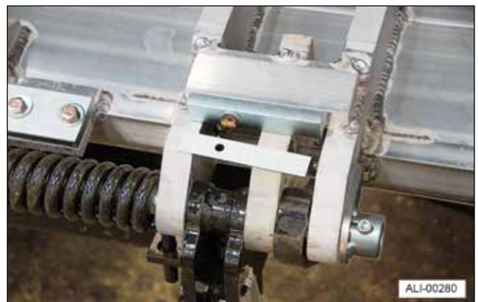
**Note:** One shim can move the ramp end of the platform as much as 1/2 inch.
