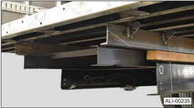
**Note:** Walk ramp stops may need to be removed. If the walk ramp is equipped with cage wheels, and they are removed, fill the open cut-outs as shown below to ensure a smooth walk ramp function.
