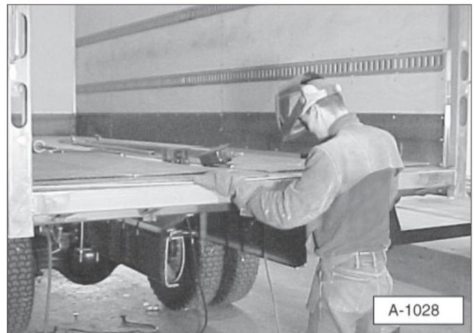
3. Lift and center the liftgate on the truck's rear sill. Make sure the top of the liftgate's housing is flush with the truck floor. The 12 inch pieces of angle iron should keep the liftgate flush with the floor of the truck.
