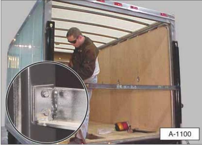
16. Cut a diagonal support brace and weld it to each H-frame rail.
