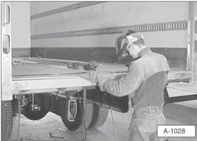
3. Lift and center the liftgate on the truck's rear sill. Make sure the top of the liftgate's housing is flush with the truck floor. The 12" pieces of angle iron should align the liftgate flush with the floor of the truck.
