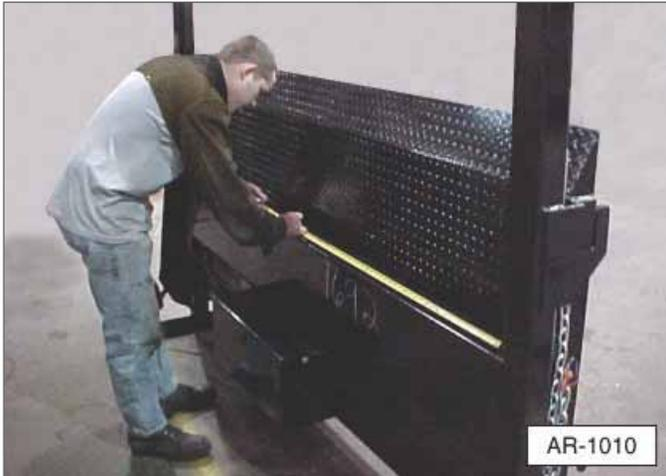
2. Measure and determine the centerline of the truck's rear sill. Mark this point.
