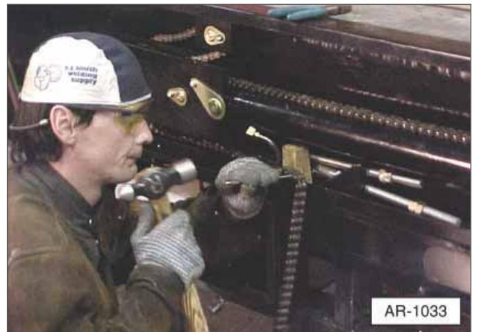
**Note:** Using a chain link removal tool will greatly reduce the time spent removing these links. These tools are normally available at motorcycle shops or other chain component suppliers.
