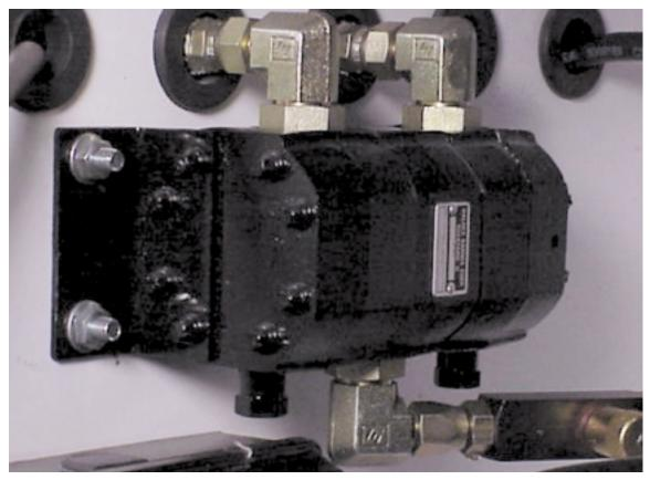
Closeup view of the Rotary Gear Flow Divider inside the Anthony Magnum RailTrac liftgate pump box with the single input flow connector (bottom) and the two output flow connectors (top). This system provides equal, self-adjusting hydraulic pressure to each liftgate cylinder.
