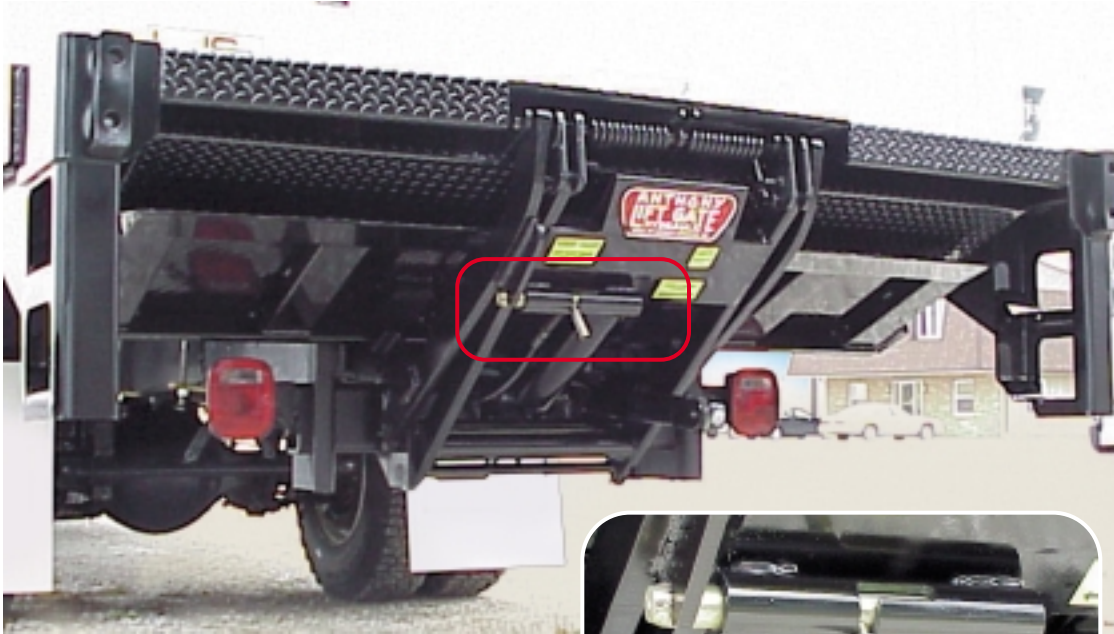
Top photo shows the ATU Tuckunder liftgate in the closed and stored position. Photo on lower right shows the new latch pin assembly. Latch pins are a Standard Feature on all Anthony Tuckunder liftgates.
